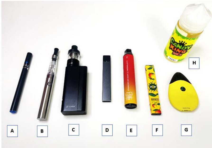
Fig. 2. Examples of current e-cigarette devices in the market. A. Blu cigalike (1st generation). B. NJOY vape pen (2nd generation). C. Vape Mod (3rd generation). D. JUUL (pod-based 4th generation). E. Puff Bar Puff Jumbo (5% nicotine salt with 2500 puffs) Strawberry and cream flavored (disposable e-cigarette). F. POP mango flavored (5% nicotine with 400 puffs) mango flavored (disposable e-cigarette). G. Suorin drop refillable e-cigarette (4th generation). H. Candy King e-liquid.
