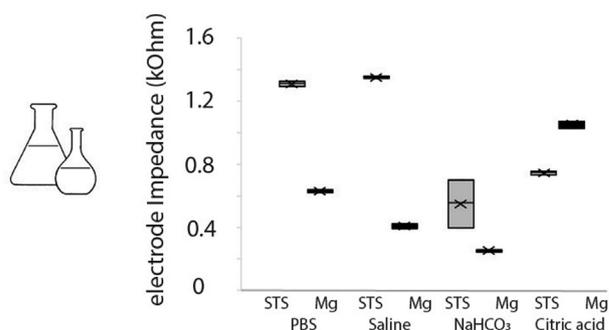
**Fig. 2 – In vitro impedance measurements with a biodegradable Mg and a nonbiodegradable stainless steel alloy electrode in different media (Phosphate-buffered saline, Normal saline, Sodium bicarbonate solution, and Citric Acid solution). Values are recorded for three separate measurements.**
