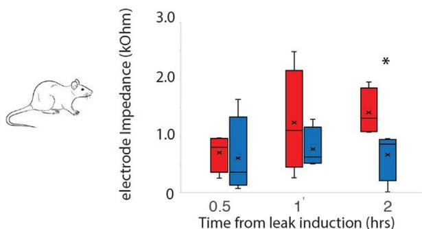
**Fig. 3 – Impedance measurements with the Mg electrode in the mouse model (Leak versus Intact tissue). n = 8, \*indicates P < 0.025.**
