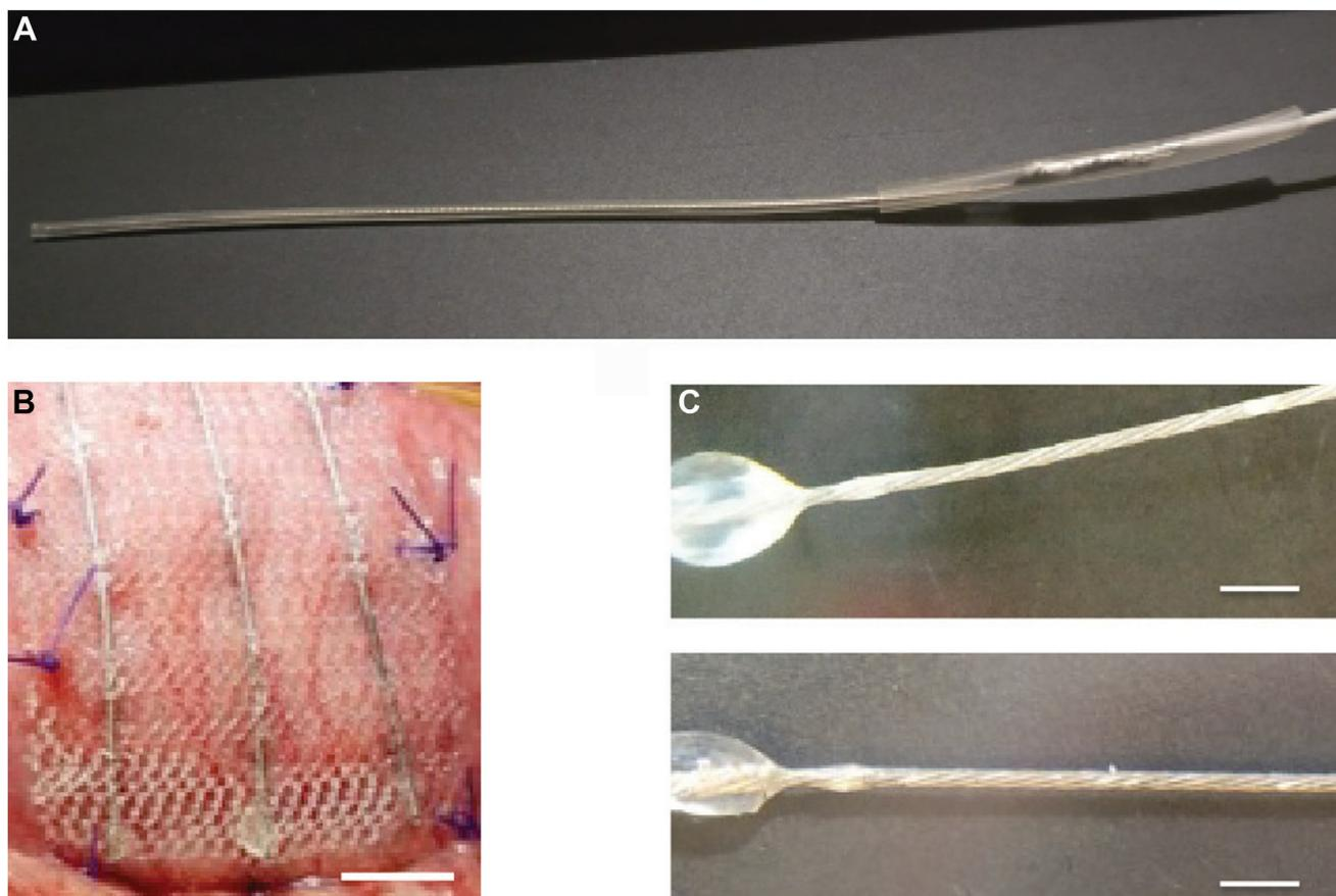
**Fig. 1 – Magnesium alloy electrode as used in the study. (A) The electrode is insulated with silicone tubing prior to implantation for *in vivo* use. (B) Three electrodes are weaved onto an absorbable Vicryl mesh for long-term implantation. Scale bar – 10 mm. (C) Active electrode before implantation (*Upper Image*) and after 7 days in physiological conditions (*Lower Image*). Scale bar – 1 mm.**
