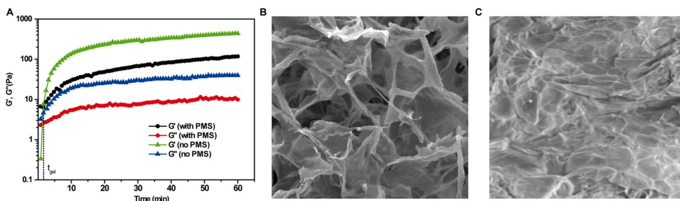
**Fig. 1 – Characterization and microstructures of CMCS/alginate-PMS hydrogels. (A) The rheological characterization of CMCS/alginate and CMCS/alginate-PMS hydrogels. (B,C) The morphology of CMCS/alginate (B) and CMCS/alginate-PMS hydrogels (C) was assessed using scanning electron microscopy.**
