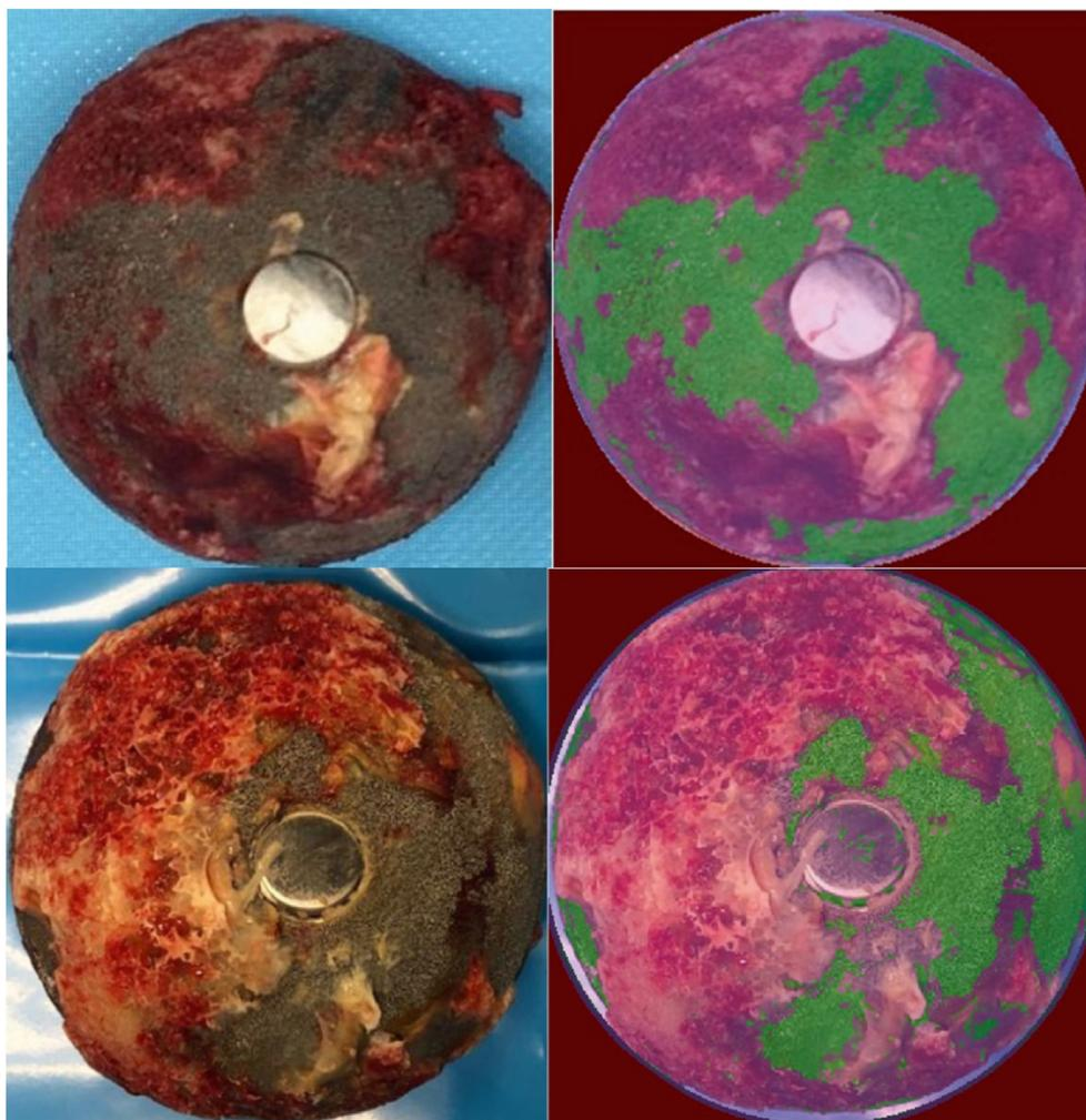
Fig. 2. Retrieved acetabular components and subsequent segmentation with ImageJ2 software.
