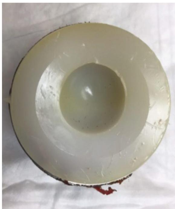
Fig. 5. Retrieved polyethylene liner demonstrating eccentric wear.
