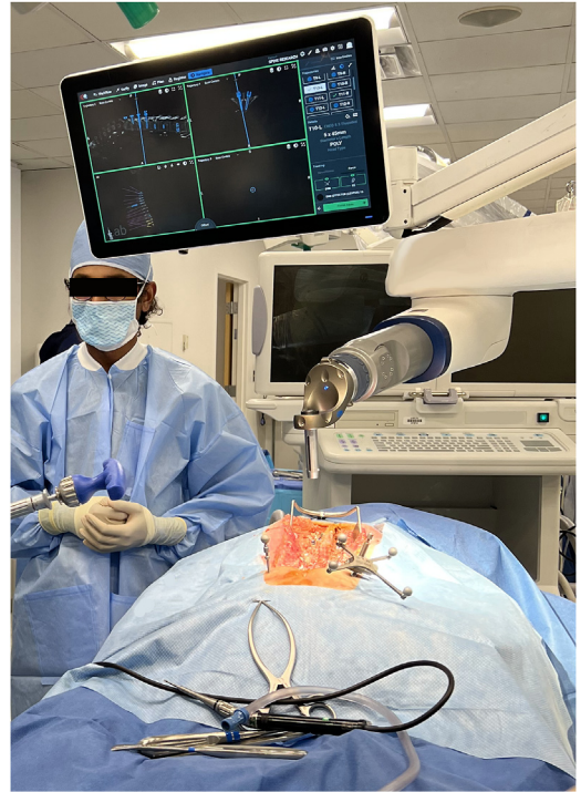
Fig. 1. An example of a surgical robot for spinal fusion surgery.
