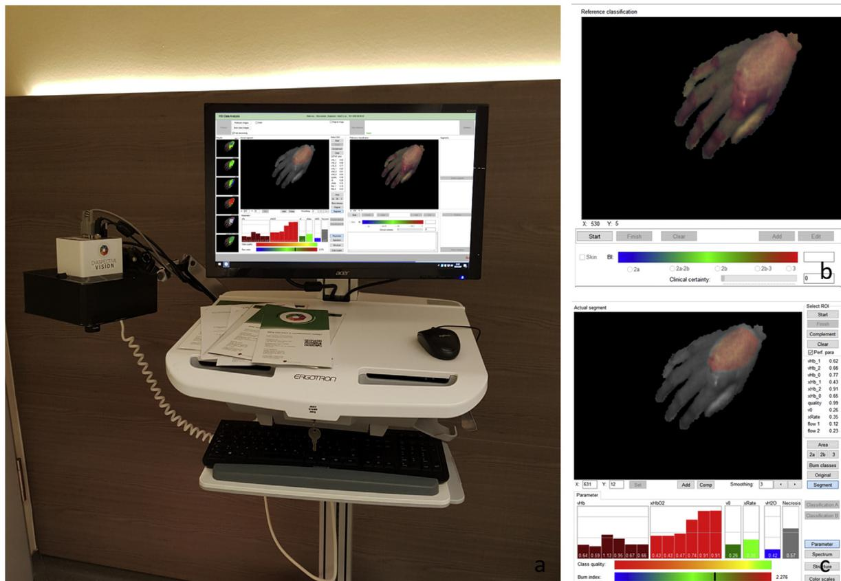
Fig. 2 – a TIVITA© Tissue hyperspectral camera. b Software system demonstrating a mixed partial thickness burns of the dorsal right hand. c After a marker is placed on the region of interest the 6-layer perfusion model including the BI is displayed.
